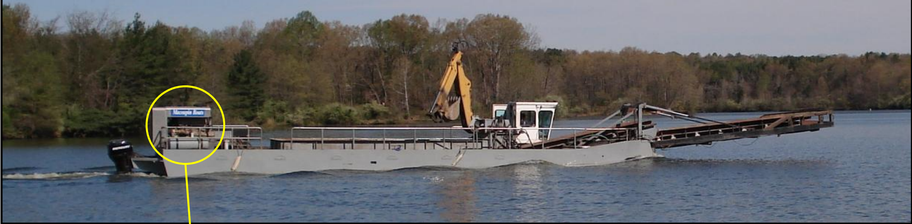
Macoupin 420 (prototype) Smaller auxiliary engine, lower bridge clearance
