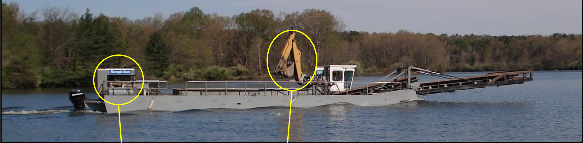
Macoupin 420 (prototype) Smaller auxiliary engine, lower bridge clearance automatic feeder replaces the backhoe
