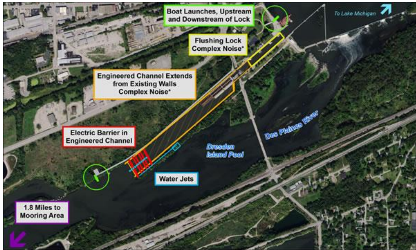
Map showing locations of key features, or measures, of the tentatively selected plan at Brandon Road Lock and Dam. [Source: USACE]
