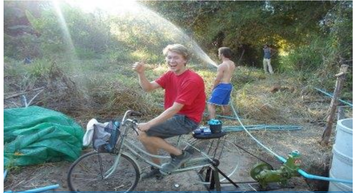
Watering with pedal power at PermaPai agriculture project in Pai, Mae Hong Son province, Thailand ( https://permapai.wordpress.com/2013/03/08/bicycle-pump-power/ )
