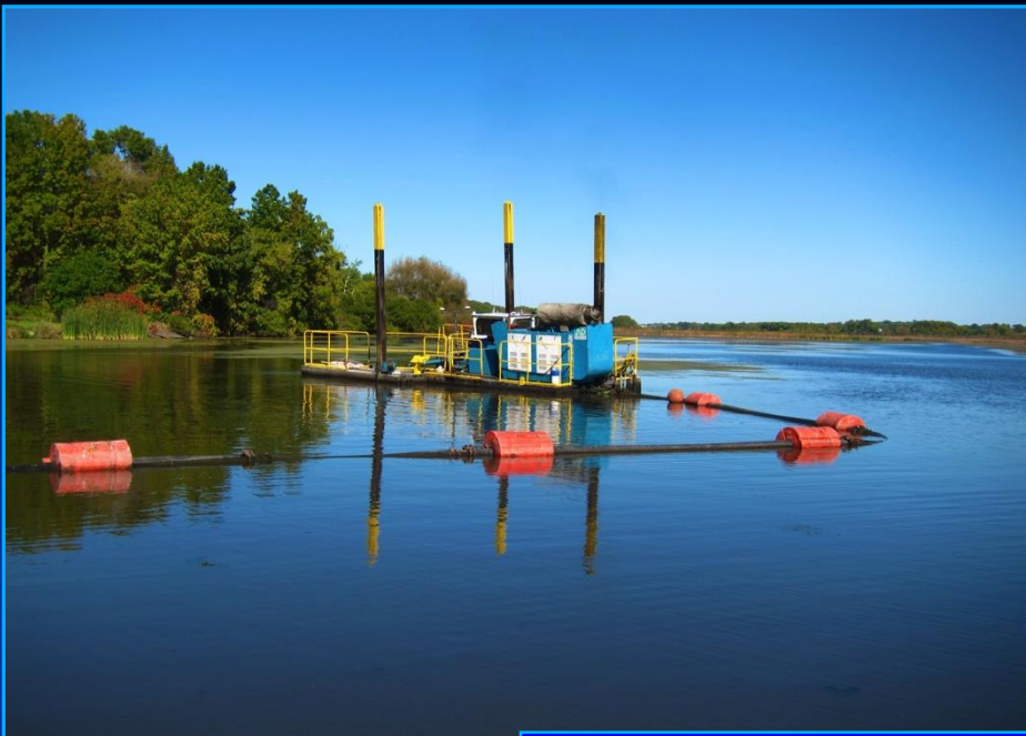
Hydraulic dredge with rotating basket type cutterhead
