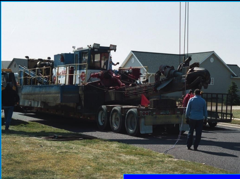
Hydraulic dredge mobilization and pipeline assembly.
