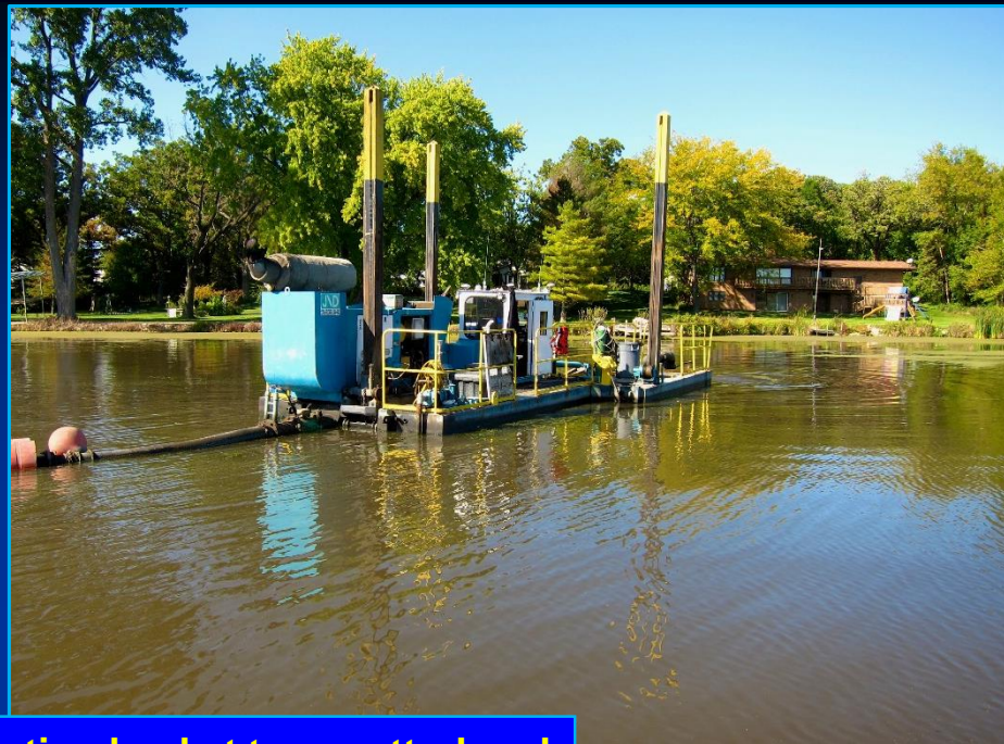
Hydraulic dredge with rotating basket type cutterhead
