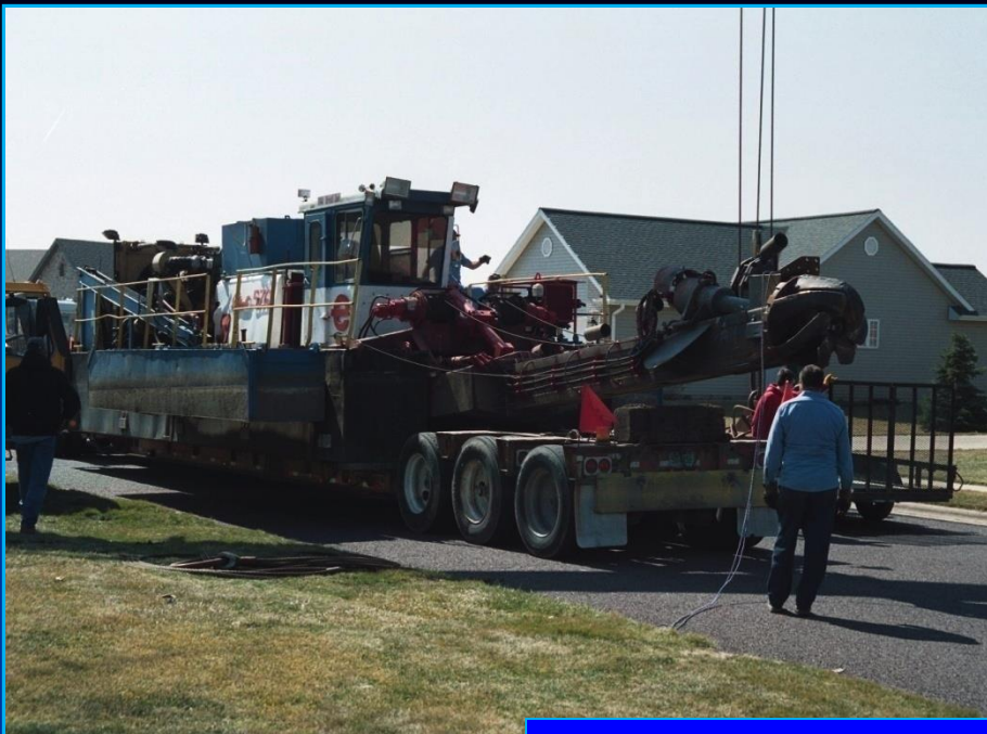
Hydraulic dredge mobilization and pipeline assembly.
