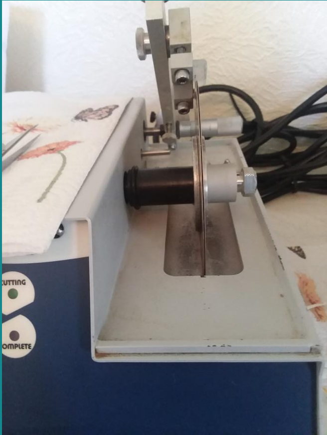
Double blade set up on an isomet low speed saw
