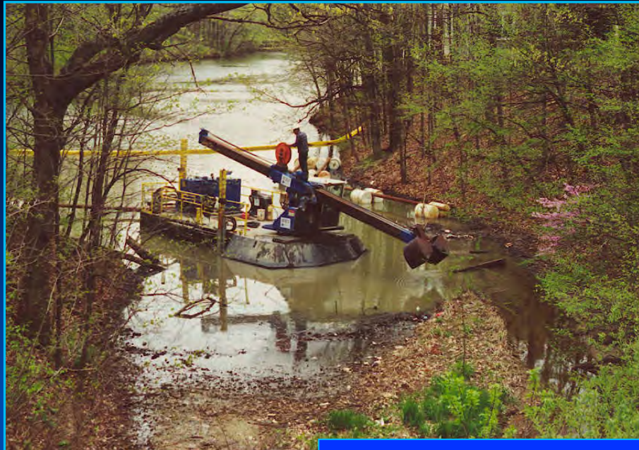
A modified high solids "Dry Dredge" can excavate material and pump a thickened slurry of "lava" consistency, which reduces dewatering and is efficient at filling geotextile tubes.
