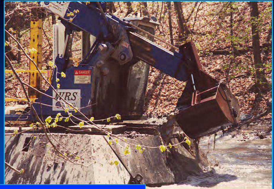
A modified high solids "Dry Dredge" can excavate material and pump a thickened slurry of "lava" consistency, which reduces dewatering and is efficient at filling geotextile tubes.
