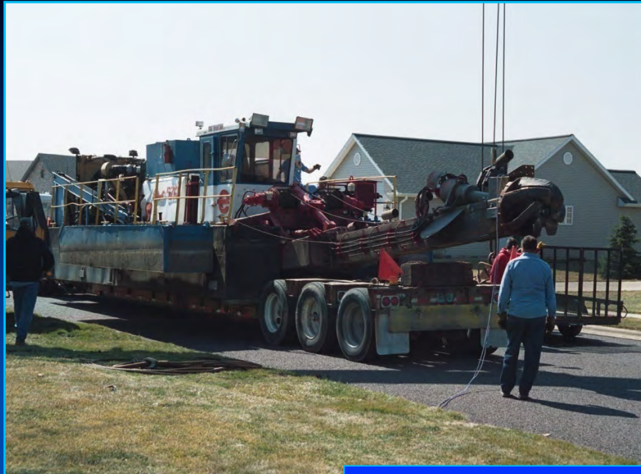
Hydraulic dredge mobilization and pipeline assembly.
