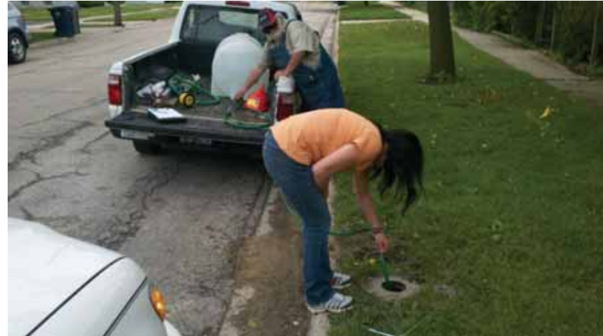
Filling monitoring well for measurement after pre-wetting 24 hrs earlier.
