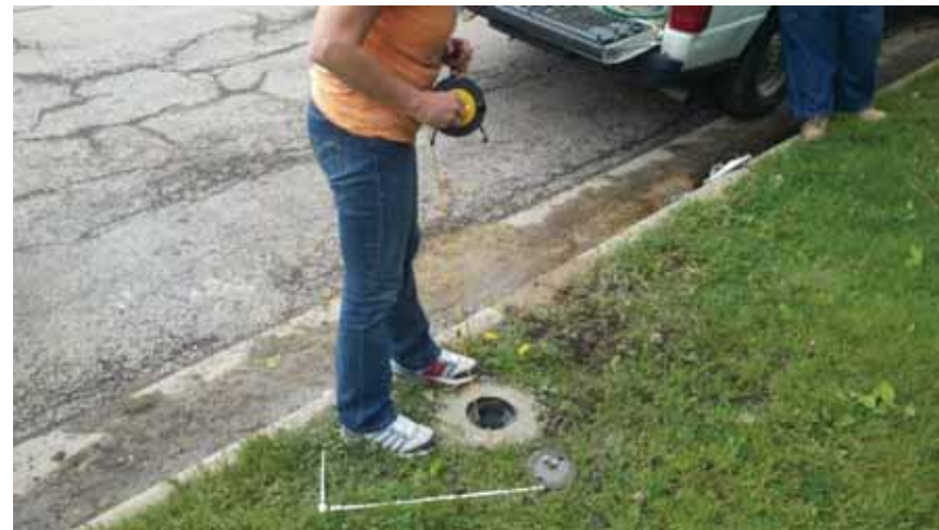
Soil boring & monitoring well installation in alley selected for permeable pavers. Measuring water level to calculate infiltration rate.
