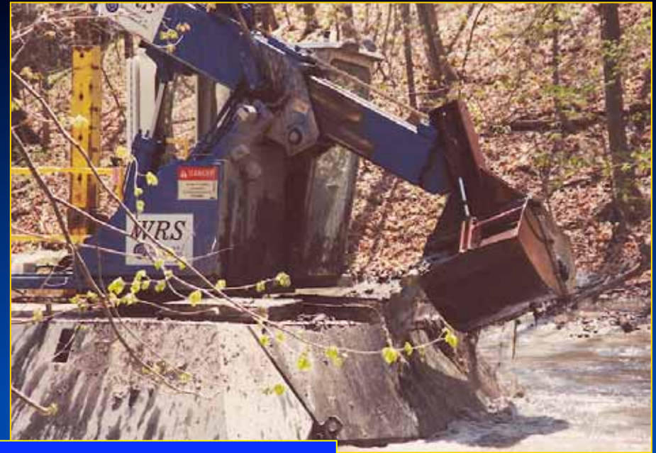
A modified high solids "Dry Dredge" can excavate material and pump a thickened slurry of "lava" consistency, which reduces dewatering and is efficient at filling geotubes.
